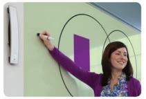
The MimioTeach bar is small, lightweight, and very durable. It snaps magnetically onto a standard whiteboard.
